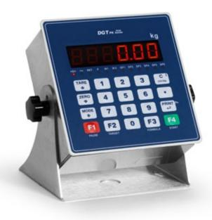
Multifunction weight transmitter for table or panel mounting. Ideal as a microcontroller in industrial weighing and dosage systems, making an easier and safer integration of the weighing to any automation system. Fitted with 4 inputs and 6 outputs, programmable. Numerical keyboard for the quick entry of the setpoint and the tare.
